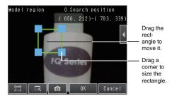
Check the area, press the [OK] Button, and then press the [TEACH] Button. The characteristic part and reference position for position compensation will be registered.
